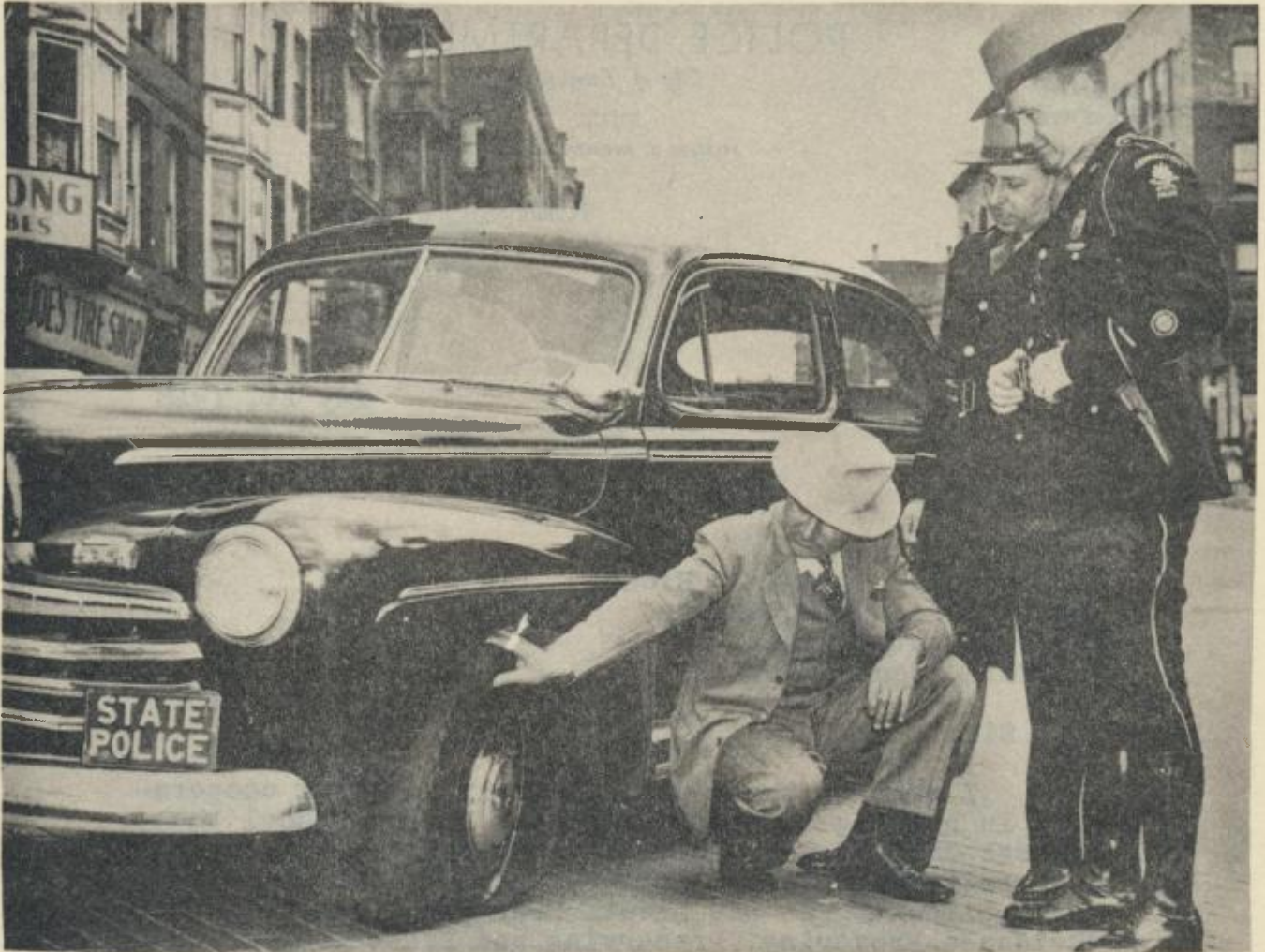
STATE POLICE inspect deflated tire after new safety device demonstration. Joseph Samoska, explains to the officers, Sergt. Leslie Williams, State Police safety division, Hartford, (left) and Officer Vincent Searles, Westport Barracks, how the new "beading" of the tire-rim prevents a tire from coming off the wheel even though the machine might be traveling as high as 65 miles per hour. The State Police car in photo is equipped with the new safety device on five wheels and will be used on patrol on the Merritt Parkway.
