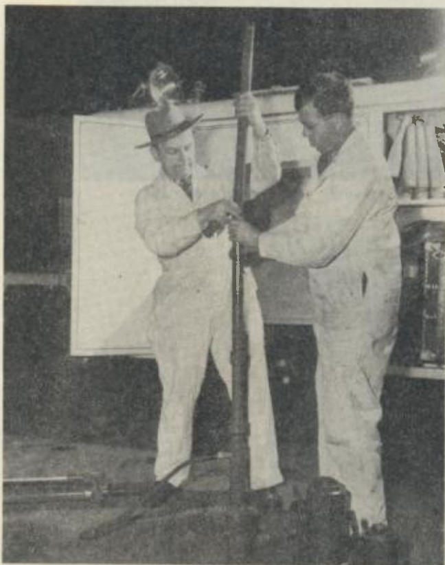
Long Jack used on wrecks can split car body, freeing victims.
